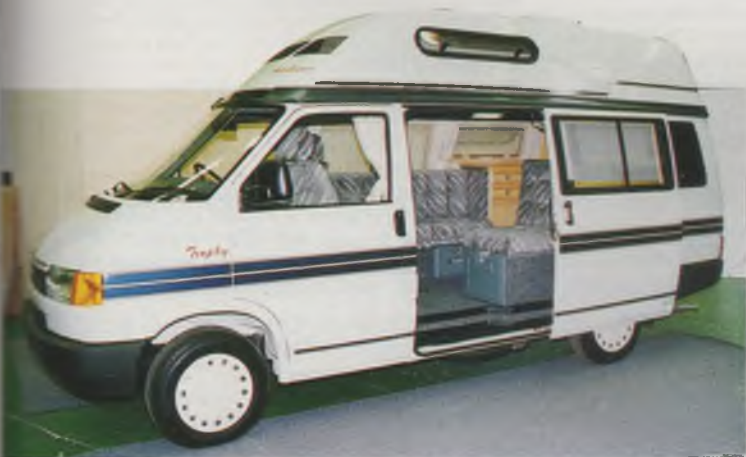
● A first view of the interior when Auto-Sleepers unveiled their prototype. Note drawer units under seats.
