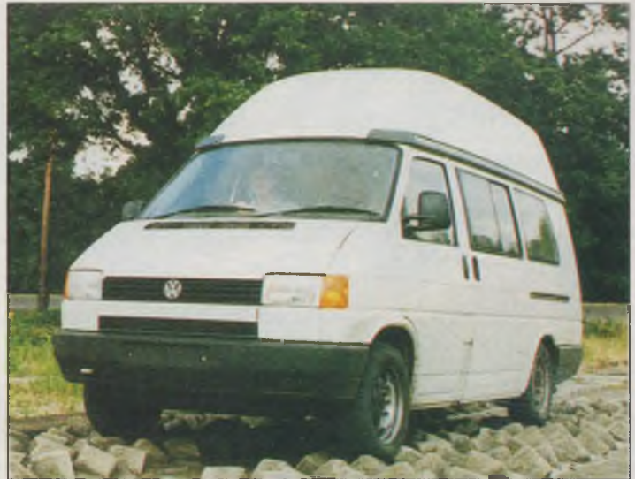
● Worst stretch of the Chobham vehicle torture trail, the randomly set kerbstones!
