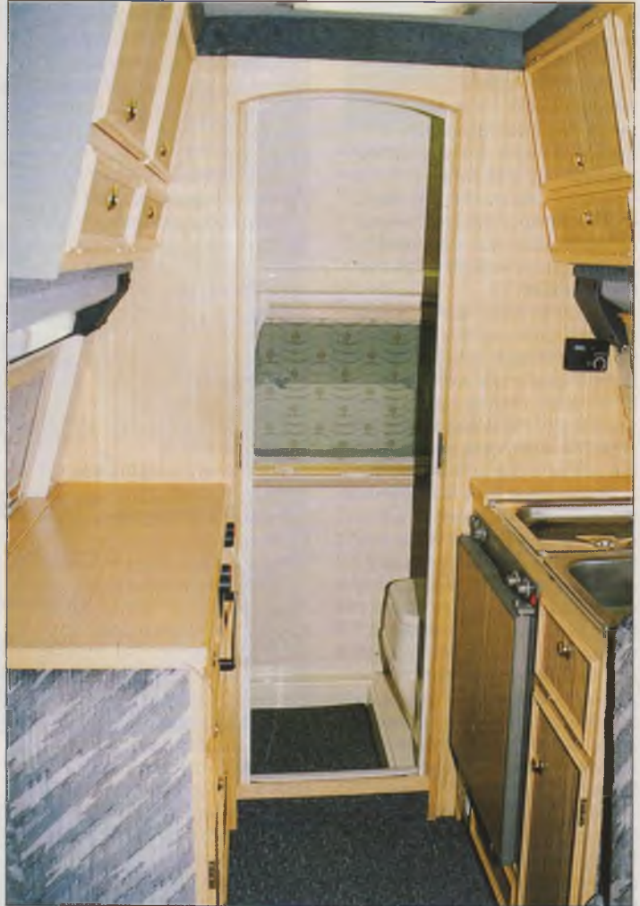
● The rear extension creates the space for a practical toilet room. To close it off, half-doors slide from both sides and thus intrude into neither toilet nor kitchen space.
