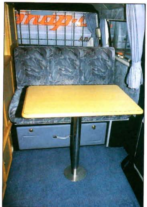
Main table caters for two sitting side-by-side on rear settee. Bench has three-point belts but no option of head restraints
