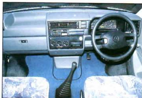
Later style T4 cab has small steering wheel, but this example is not new enough to have the larger instrument dials with striking blue illumination
